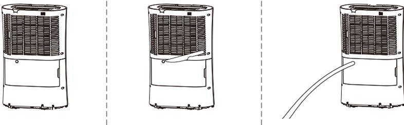
Make sure the connection between pipe and the drain outlet is tight and does not leak. Then direct the pipe to a suitable drainage point. This unit uses gravity to dispose of water hence the drain should be lower than the water outlet on the unit. Put the tank back. Be sure to run the water pipe downward and let the water to flow out smoothly. Do not kink or bend the pipe.
