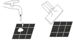
Remove the ABS filter frame. If the optional carbon filters are fitted, remove them from the frame and Hoover gently approximately every 2-3 weeks.
